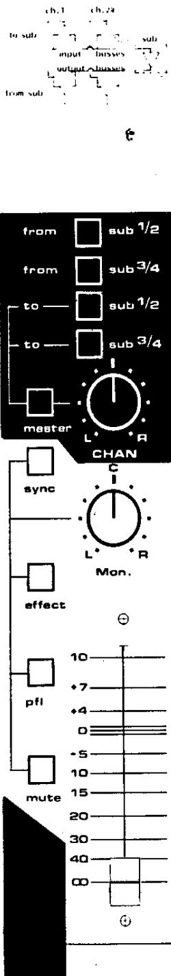
multitrack inputs to the outputs of the subgroup amps. This is done by switching the "from sub 1/2" switches. As you can see it is very easy to bring this signal to any multitrack input or even more than 1 multitrack channel, if you like.
