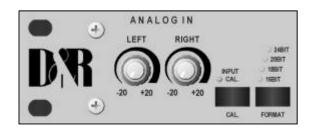
The analog input offers separated level control of the left and right channel. When the CAL. indicator is illuminated, the input level can be adjusted via the controls on the front panel. When the input CAL is off, the gain controllers are disabled and the level is set to the studio's standard headroom level. This level is set by means of internal trimmers.
