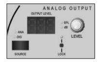
The analog output is operated in the same way as the digital outputs. The source select enables you to address either the digital-or analog input.
