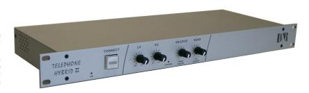
A large ring button enables you to pick up the line from the unit itself or from your mixer when connected via its GPIO to the telephone Hybrid. Both levels of receive and send can be adjusted to suit your requirements. Incoming signals can be tailored by the variable high and low cut signal while talking to people calling the station. A ducking system reduces the incoming signal while talking to people calling the station. Input and outputs on XLR's, jack, 9 pin Sub-D and RJ-11 connectors.
