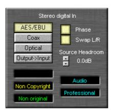
The 'Source Headroom' is a very useful function. This setting give's an indication of the headroom, which is used, at the applied audio signal. The Sirius system is now able to make a correction to the internal nominal headroom level.
