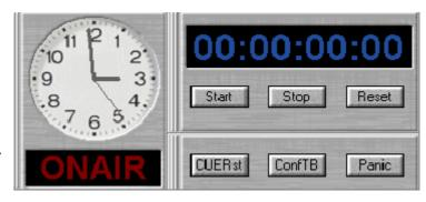
button or by assigning the Timer to a fader-start (see 7.2 Input and output ) The Stop knob stops the Timer when started by the Start knob or fader-start. The Reset button shall reset the Timer to 00:00:00:00
