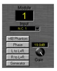
When you are ready with selecting the input sources you need for the job, you can now trim your input level with a range of 40 dB (-20dB to +20dB) by way of the input gain potentiometer. This can be done on screen or on the gain motor potentiometer in the Super module, as is the case with the phase reverse switch.
