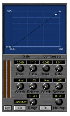
The Range control adjusts the amount of attenuation when the gate is closed An On/Off switch is implemented.
