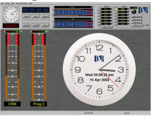
All main output meters show also a phase meter, which indicates mono compatibility. The phase meter is a center zero type. A perfect stereo signal will show 0, which is random distributed phase. A Mono signal will be indicated with +1 and an out of phase signal by -1. As long as the pointer moves within the green section the signal is mono compatible (sufficient in-phase components) when the pointer is in the red section the signal is not mono compatible (to much out of phase components).
