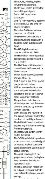
A smooth feeling K-Alps fader (P&G is optional) with optional faderstart switch completes the channel.
