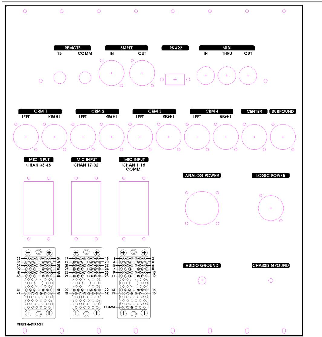
The master backpanel houses the remote connectors for the Talkback and Communication mics, balanced SMPTE in and out XLR's, an RS 422 computer connector and the Midi in, thru, and out din type connectors.
