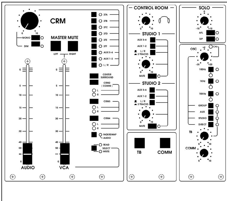
If you would like to build up a mix from one of the stereo Aux pairs, press the **L/R - 2 TRACKS** switch and make sure no stereo machine is routed in the stereo source switches. Both studio outputs can be muted. Studio 1, 2, or both can be used for stereo headphone feeds or studio playback speakers.
