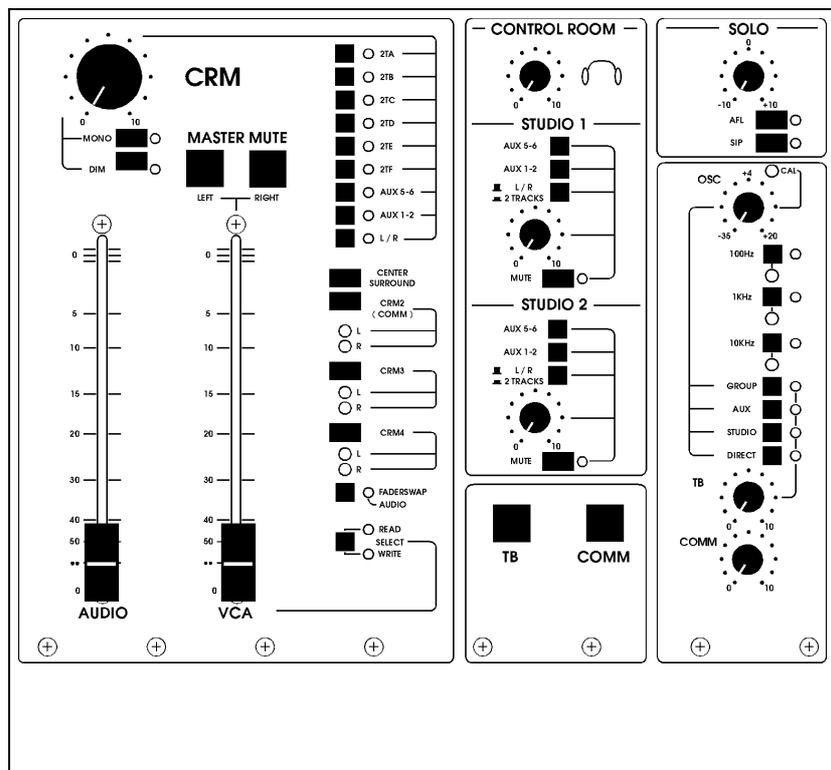
The oscillator can be assigned to the Group busses, Aux busses, Studio outputs, as well as the direct output (in the patchbay). Each of the oscillator assignment switches have an led indicator. The CRM will dim 20dB when the oscillator is active.
