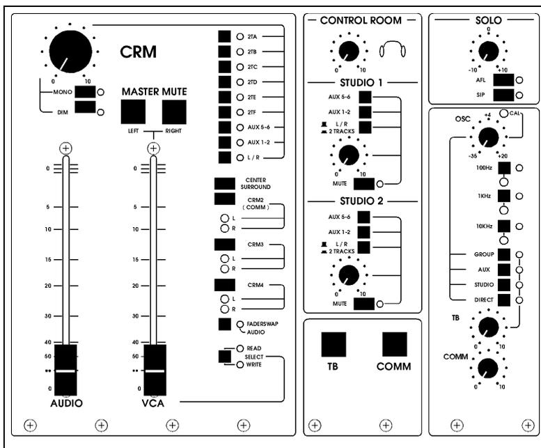
The large CRM knob controls the total outgoing level to the control room monitor power amps. This control is a quad device.
