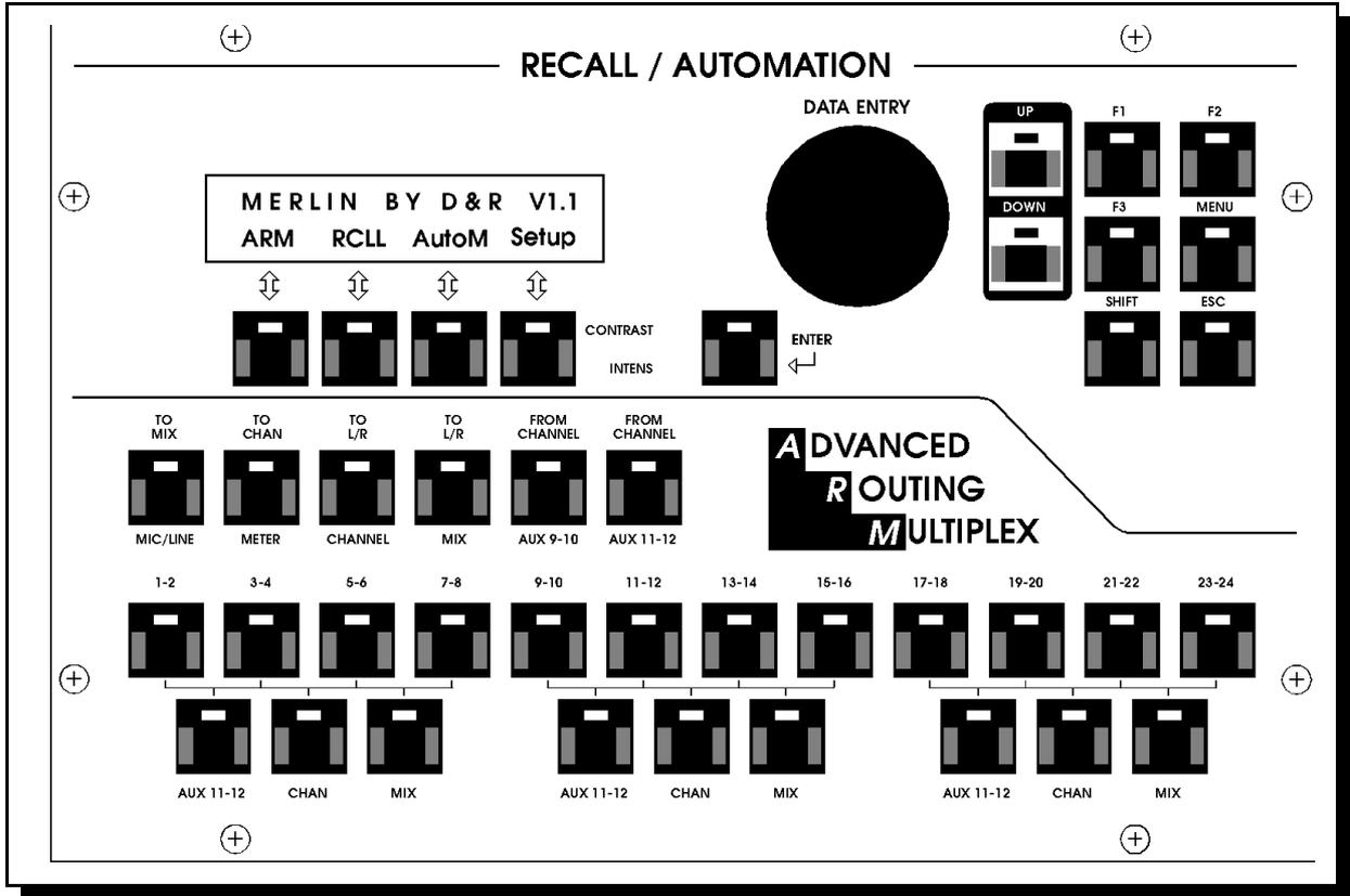
If you press the **S3** switch below the LCD (when it's showing **STORE**) these settings will be stored for the module that has its' **ARM** light on.
