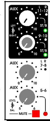
Aux 5 through 8 are always in the CHANNEL path. Aux 7 - 8 are dual concentric controls with 7 being the top knob and 8 the bottom knob. The top knob on Aux 5 - 6 is a level control and the bottom knob is a balance control. The balance control is used to balance the stereo signal and not a pan pot.
