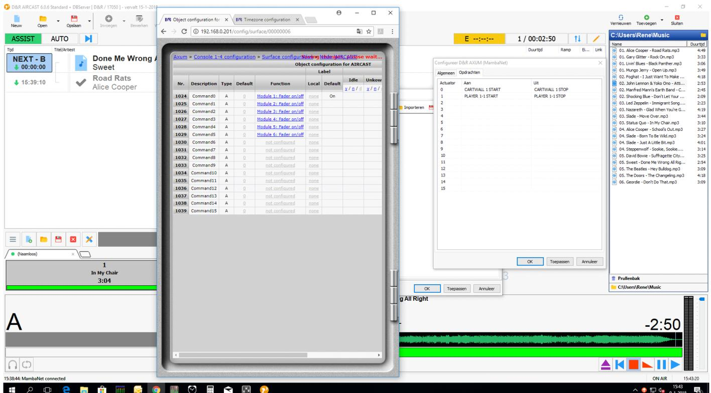
This image shows how the fader of module 1 and fader of module 2 of the Axum can activate and stop a Cartwall player and player one.
