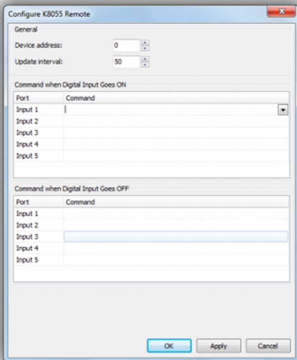
First, you can set up the **device address** (corresponds to the jumpers on the board) and the **update interval** for polling.
