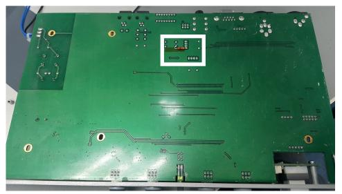
solder a 1 kOhm 1 watt leaded resistor on the bottom side of the pcb between the + pin of C16 and Pin 6 of TR 1 See picture on the left.
