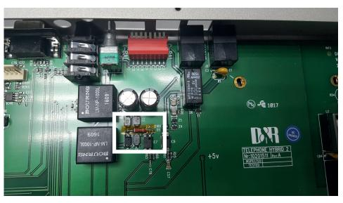
Solder a 620ohm 1W leaded resistor in between the cathodes of D3/4 and Pin 1 of IC 7
