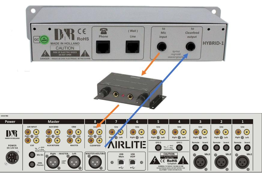
For an Airlite connect the Cleanfeed output of the Airlite to the to cleanfeed output at the Hybrid-1
