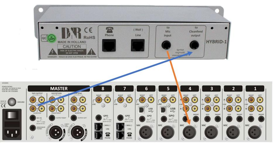
For an Airmate connect the Cleanfeed output of the Airmate to the to Cleanfeed output of the Hybrid-1.
