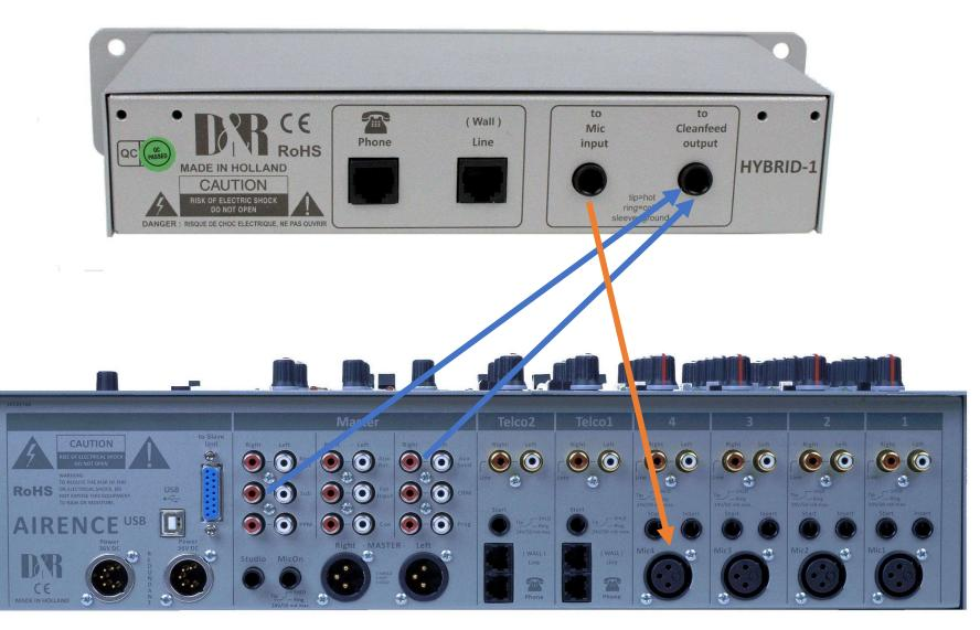
For the Airence connect the Sub or Aux send of the Airence Main to the "to Cleanfeed" output of the Hybrid-1. Connect the to Mic input of the Hybrid to a Mic input at a desired Channel of the Airence Main or Airence Extender. Set the Sub or Aux send of all the other channels to "On" and the channel where you connected the Hybrid-1 at to "Off".
